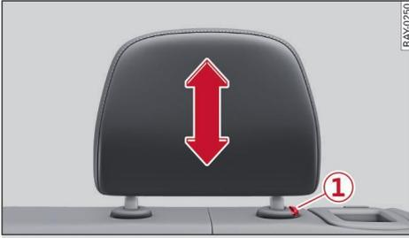
Fig. 33 Rear seat: Adjusting head restraint
