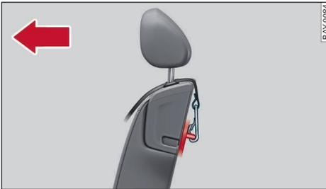
**Fig. 46** Rear backrest: Hooking strap into top tether anchorage
