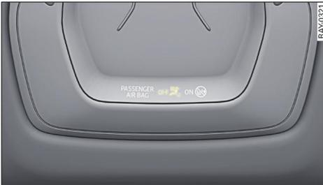
Fig. 41 Headliner: Indicator lamp for status of front passenger's airbag
