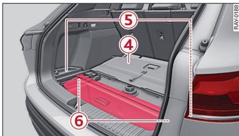
Fig. 51 Luggage compartment: Stowing the luggage compartment cover underneath the floor panel
