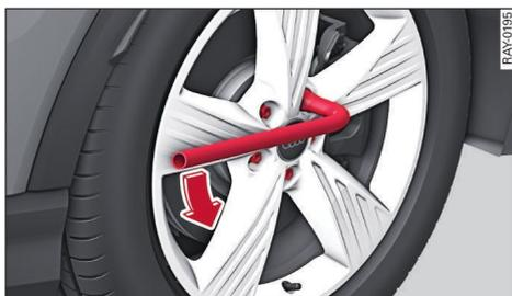
Fig. 136 Wheel: Loosening the wheel bolts
