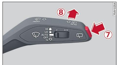
Fig. 24 Control lever: Rear window wiper
