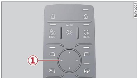
Fig. 20 Driver's door: Control panel for exterior mirrors
