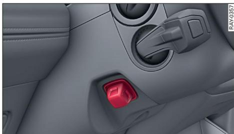
Fig. 30 Steering column: Button for adjusting the steering wheel position
