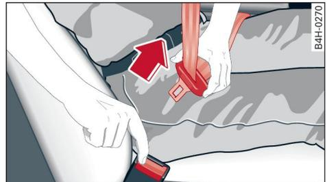
Fig. 38 The latch plate of the belt springs out of the buckle
