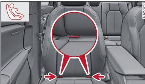
Fig. 44 Front passenger's seat: Bottom ISOFIX anchorages
