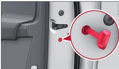
Fig. 6 Door: Locking the door manually
