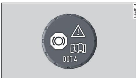
Fig. 125 Front compartment: Cap of brake fluid reservoir
