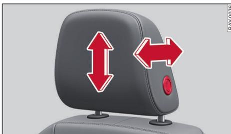
Fig. 32 Front seat: Adjusting head restraint
