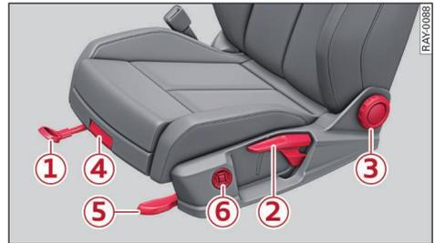
Fig. 27 Front seat: Adjuster controls
