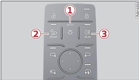
Fig. 15 Driver's door: Light switch module
