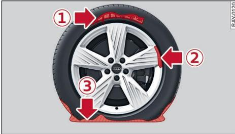
Fig. 131 Tyres: Irreparable tyre damage
