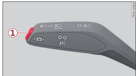
Fig. 91 Turn signal lever: Button for lane guidance and lane departure warning
