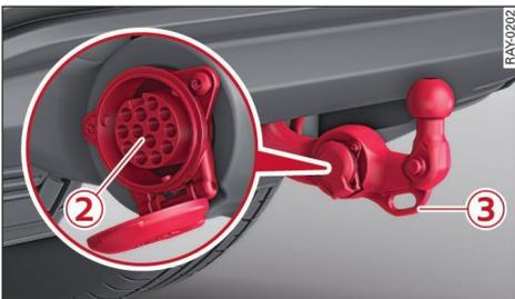
Fig. 73 Rear bumper: Connecting socket and eye for breakaway cable
