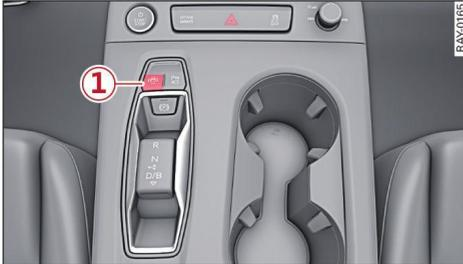
Fig. 82 Centre console: Button for driver assist systems
