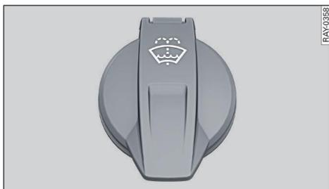
Fig. 128 Front compartment: Cap of windscreen washer container
