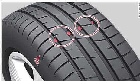
Fig. 129 Tyre tread: Tread wear indicators
