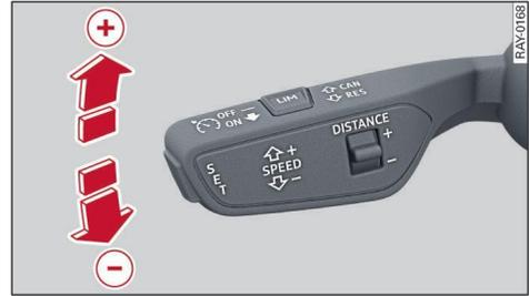
Fig. 98 Control lever: Setting a new speed
