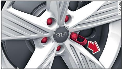
Fig. 134 Wheel: Wheel bolts with caps
