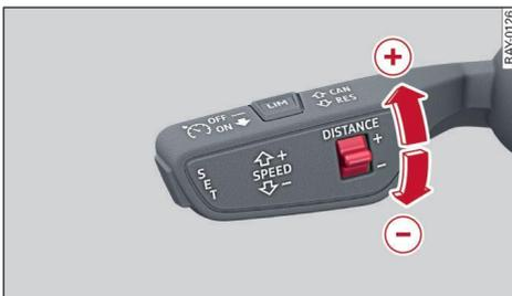
Fig. 99 Control lever: Setting the distance
