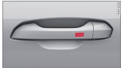
Fig. 9 Door handle: Sensor for locking the vehicle
