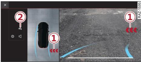
Fig. 113 Centre display: Rear cross-traffic assist display
