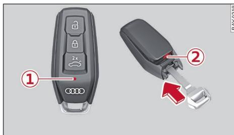
Fig. 8 Vehicle key: Removing battery cover
