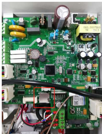
MicroSD slot of 7kW charger
