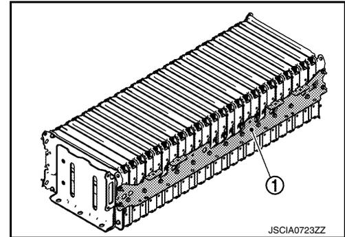
5. Fasten the rear module stack ① with a lashing belt ②.
